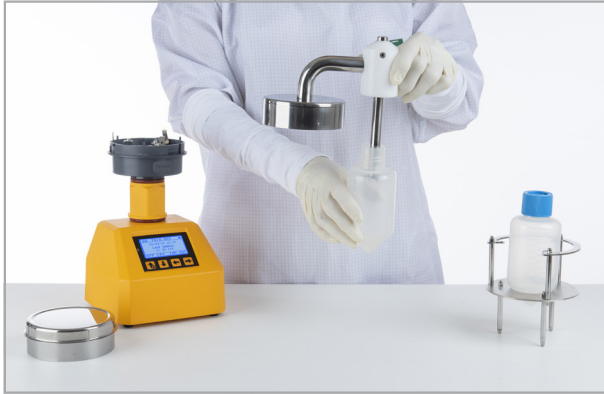
3. Take out the conical tube from the collection liquid system
