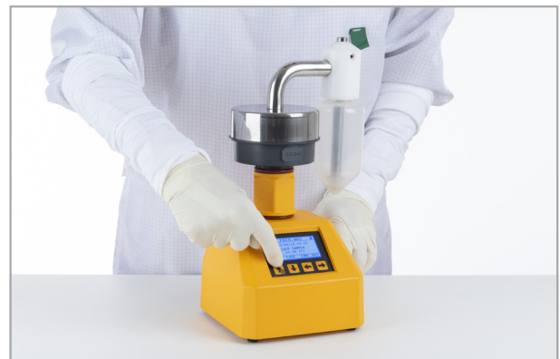
6. On the air sampler, select VIRUS under SPECIAL SAMPLING menu and press START
