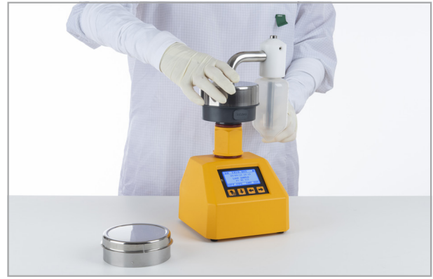
2. Position the collection liquid system into the AIRBIO ONE RAPID-VIRUS
