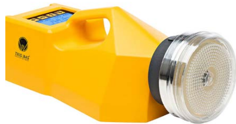
6 - TRIO.BAS MONO System ready for sampling
